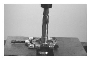
**18.** Remove the **outer** roller bearing. Use a knife extractor as a counterhold, with a **17 mm** socket on the shaft end.
