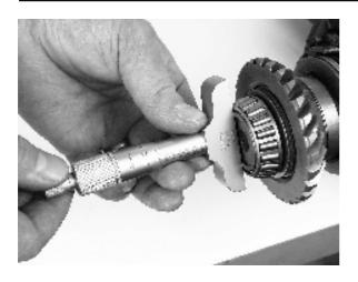
34. Install the sintered washer and press the bearing on.
