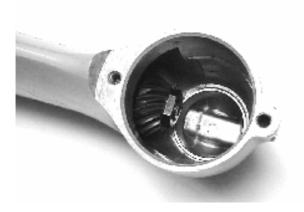
**42.** Install the vertical shaft in the housing. Be careful to ensure that the needle rollers do not fall out. Then install the pinion. Apply thread locking fluid, Volvo Penta part no. 1161075-5, on the threads and install the nut.
