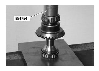
29. Press the outer roller bearing down onto the propeller shaft. Use mandrel 884754.
