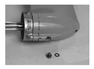
70. Change the gasket on the oil drain plug.
