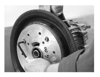
**4.** Remove the adapter plate and remove the rubber sleeve.
