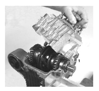
85. Install the shaft seal (1).
