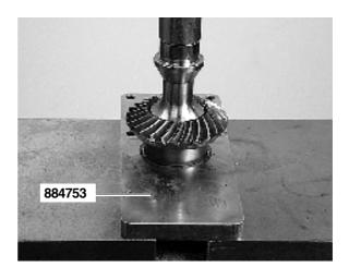
**21.** Press the gear wheel down to the step on the propeller shaft with tool no. **884753**. Make sure that it seats securely.
