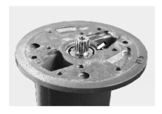
**62.** Install the calculated thickness of shims and gasket on the division plane of the lower gear housing. **NOTE!** The text on the gasket must face upwards. The hole pattern in the gasket only fits one way round.
