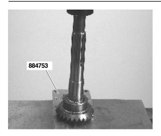
**19**. Disassemble the gear wheel with tool no. **884753**. Use a socket to protect the end of the shaft.
