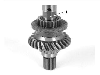
30. Install the flange, complete and key (1).
