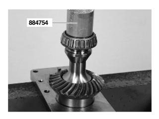
22. Install the inner roller bearing with tool no. 884754.
