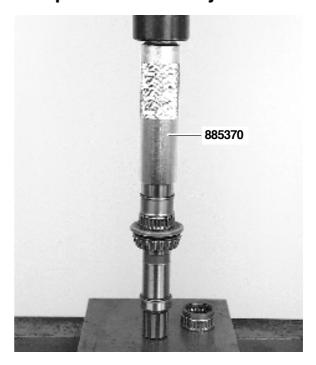
28. Press the bearing – sintered washer – needle roller bearing – spacer – needle roller bearing race on. Use mandrel 885370. Make sure that the components seat securely.
