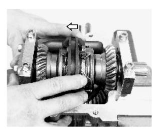
**43.** Engage the gear position for the gear wheel to be checked, by sliding the gear selection plate towards the wheel as in the illustration.
