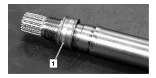
12. Remove the ferrule (1). Use a knife puller as a
