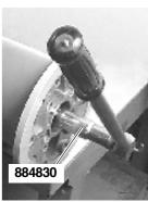
**43.** Lock the pinion nut with tool **385885.** Press the shaft down and make sure that the pinion nut engages in the tool. Fix the tool to the rear bearing housing, using socket cap screws.
