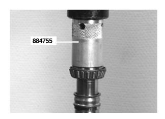
15. Install a new roller bearing with mandrel 884755.NOTE! Press until the bearing just touches the ferrule.
