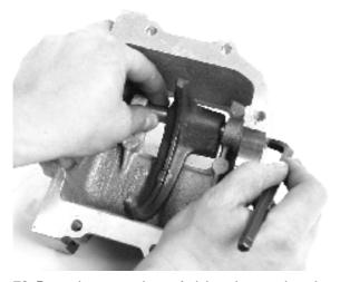
**76.** Press the gear selector fork into the gear housing. Please refer to the illustration.
