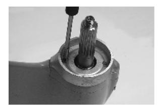
69. Install a new zinc ring. Tightening torque: 12 Nm (8.8 lbf-ft)
