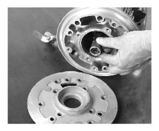
**6.** Remove the splined sleeve. Check that the sleeve is not damaged.
