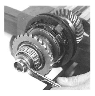
4. Fix the input shaft in a vise. Use soft facings on the vise jaws.
