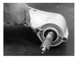
44. Install the bearing housing on the propeller shaft.
