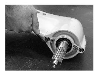
**3.** Remove the two socket cap screws in the bearing housing.
