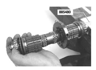
**15.** Put the components on the "measurement shaft", special tool **885480** as in the illustration. Bearing – sintered washer – needle roller bearing – spacer – needle roller bearing – spacer – shim – flange – hub – shim – spacer – needle roller bearing – spacer – needle roller bearing – flange – sintered washer – bearing – washer – screw.
