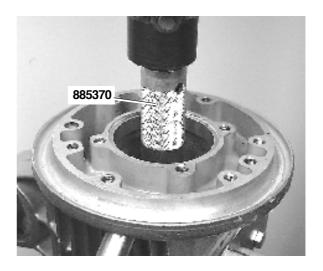
67. Press the bearing race in with tool no. 885370.
