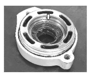
**36.** Put shims of the correct thickness in the bearing housing. In this case, they are 0.45 mm (0.0177") . Please refer to item 32.
