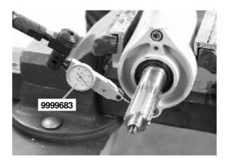
**48.** When the highest torque specified above has been reached, the gear housing should be removed from the vice and fixed vertically instead. Let the tool remain on the gear housing.
