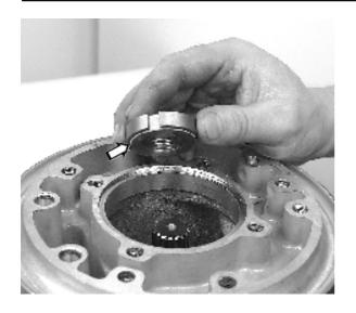
**68.** Install the ring nut. **NOTE!** Location of nut (edge).
