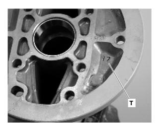
**25.** Dimension (**T**) is stamped on the starboard side of the gear housing division to permit the shim thickness under the inner bearing race to be calculated, which is 17 in this case. The dimension of the division plane can vary between 0 and 30.
