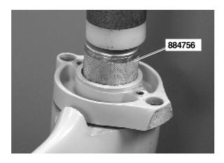
28. Install the inner bearing race in the gear housing with mandrel 884756. Use the rear bearing housing as a guide.
