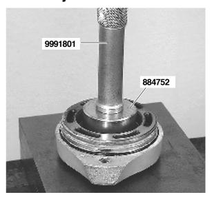
**33.** Install a new seal ring in the bearing housing, using tool no. **884752** and shaft **9991801**. Apply sealant, Volvo Penta part no. 1161099-5, to the mating face between the seal and the bearing housing.
