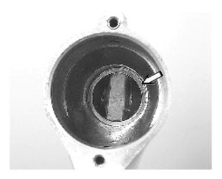
**27.** Put shims of the correct thickness in the lower gear housing. Add a further 0.05–0.10 mm (0.001968–0.003936"). In this case, we put a total of 1.00 mm (0.03937") shims in the housing.
