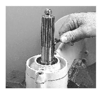
38. Install the propeller shaft in the gear housing.
