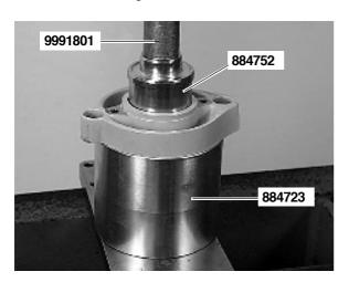
**20.** When the seal rings are changed, the outer bearing race should also be changed.
