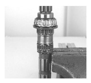
**6.** The bearing – sintered washer – needle roller bearing – spacer – needle roller bearing – spacer – shim and key are left on the shaft.
