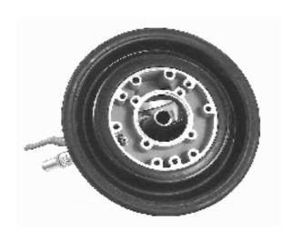
**63.** Put the rubber sleeve on the upper gear housing. Install the cooling water tap. Apply sealant, Volvo Penta part no. 1141570-0 on the threads.
