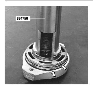
**37.** Assemble the outer bearing race with tool no. **884756**.
