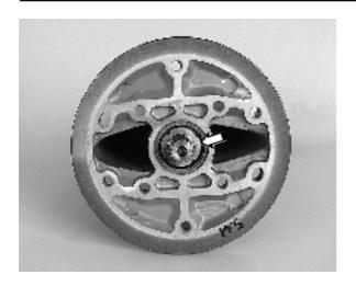
**45.** Install the upper nut on the vertical shaft. **NOTE!** The chamfered side of the nut must face downwards.
