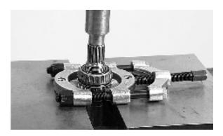
11. Remove the roller bearings with a knife extractor as counterhold. Use a hydraulic press together with a suitable mandrel.
