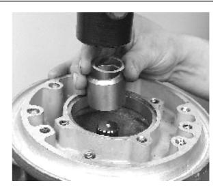
**66.** Insert the shaft, spacer sleeve and shims with thickness calculated as in item 64.
