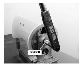
**47.** Install tool **884830** on the vertical shaft. Turn the shaft clockwise with a heavy wrench or torque wrench. Wrench size: **17 mm**.
