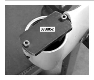
**5.** Lock the pinion nut with tool no. **3858852.** Press the shaft down and make sure that the pinion nut engages in the tool. Fix the tool to the rear bearing housing, using socket cap screws.
