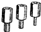
Main bearing cap remover (basic tool) 18G42A Main bearing cap remover adaptor 18G42B
