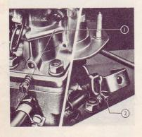
Fig. 8 Carburettor Slow-running Adjustment
