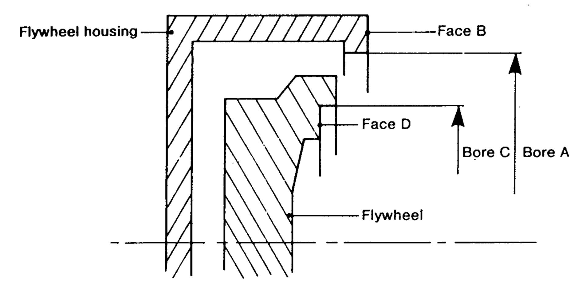
Fig. 7. Checking engine flywheel and flywheel housing.
