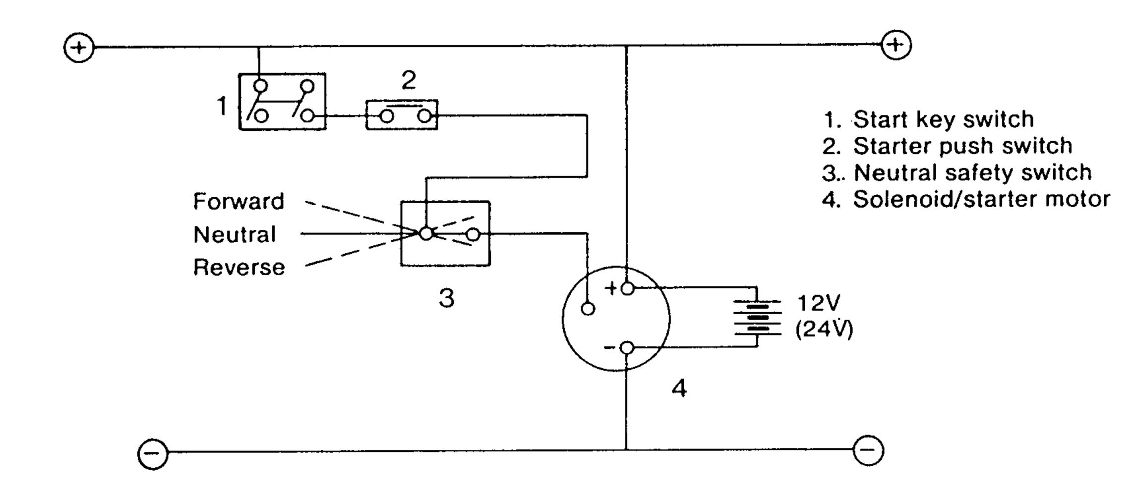
Fig. 3. Wiring Diagram for Neutral Safety Start Device.
