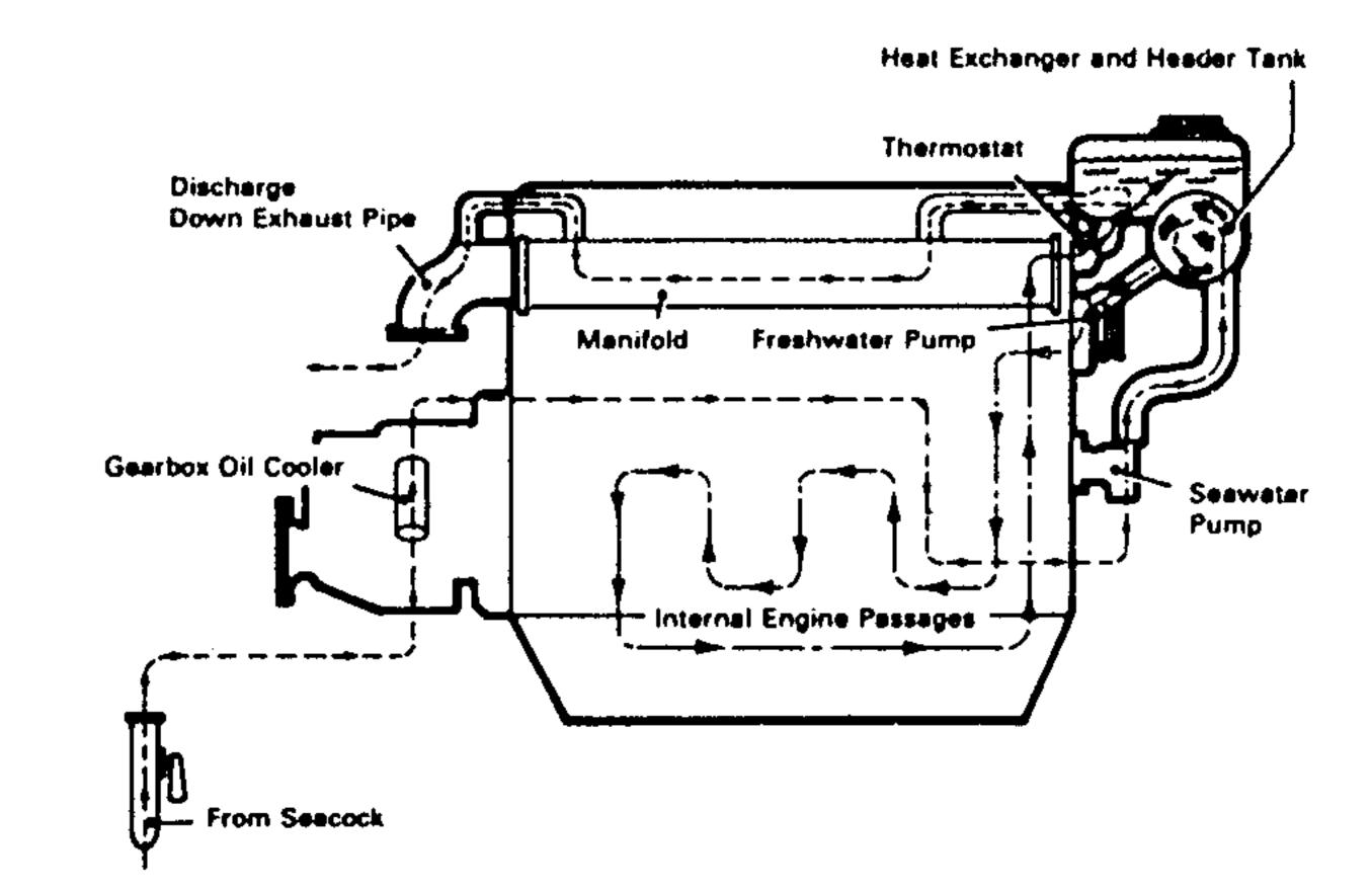
Fig. 8. Gearbox and Engine Cooling Circuit
