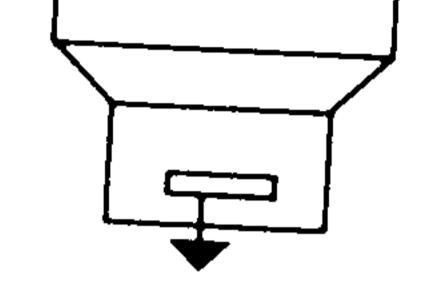
Port Engine Lever Forward L.H. Propeller Rotation
