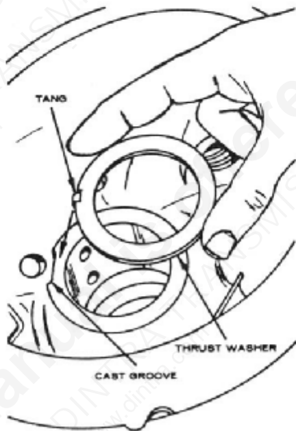
FIG. 9 THRUST WASHER USED FOR 2.10 REDUCTION UNIT
