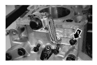
34. Flywheel with cover and coupling. Unscrew the hot water outlet (1).
