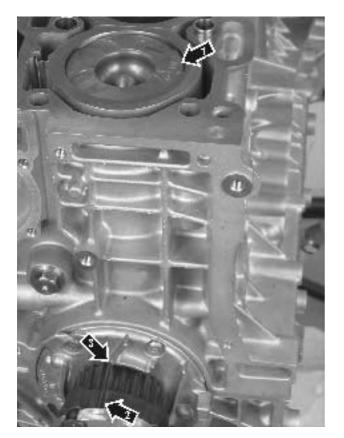
2. Crank the engine clockwise until the crankshaft locks. Be careful to ensure that it is locked in the correct position.
