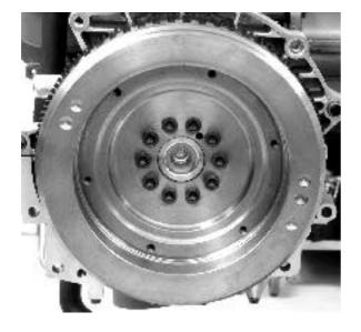
37. Unscrew the flywheel, using 12-tooth bit 885823 and remove the flywheel.
