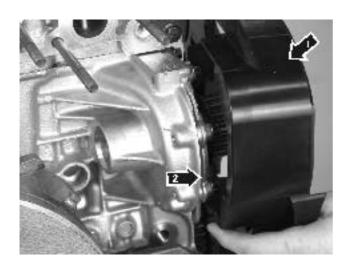
Install the rear timing gear cover (1). Check that it comes into the correct groove (2) behind the coolant pump.
