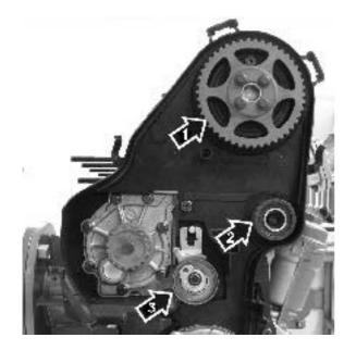
12. Remove the camshaft gear (1), jockey pulley (2) and belt tensioner (3). Remove the rear cover.
