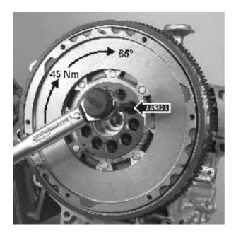
8. Install lock pin 9997005 for the crankshaft in the engine block, please refer to "Engine, disassembly, timing gear".
