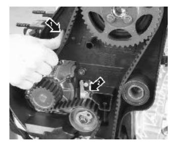
39. Apply pressure (1) to the toothed belts and check that the belt tensioner (2) moves.
