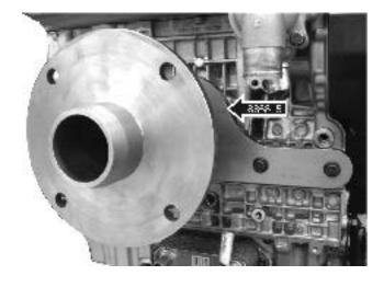
6. Install engine fixture 885815 on the engine. Set the engine up in stand 9986485.
