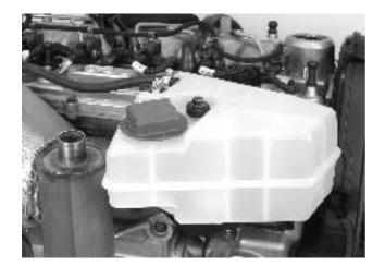
55. Install the expansion tank on its bracket. **NOTE!** Do not forget the spacer tube for the fixing screw.
