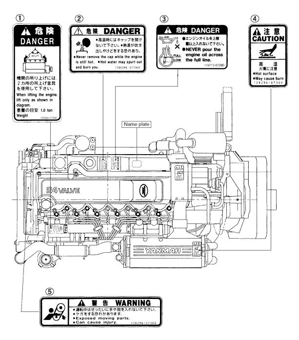
The above illustration shows an overhead view of the engine.
