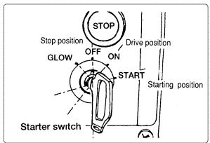
**GLOW** is the position for heating the glow plug. The glow plug is heated before starting to warm up the intake air and to aid starting during cold weather.
