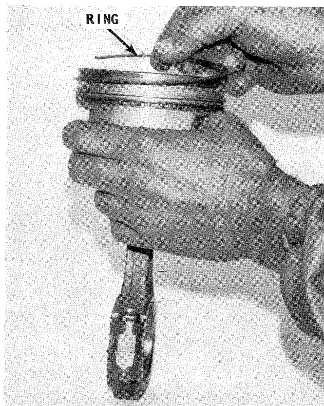
Proper installation of a new ring into the piston ring groove. Notice how the ring is bent slightly upward (left). After the ring is started, the ring is rotated around and over the top of the piston (right). The ring will feed into the groove and the end will finally snap into place.
