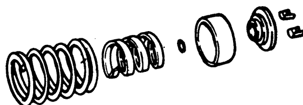
Arrangement of valve mechanism parts before and after installation.
