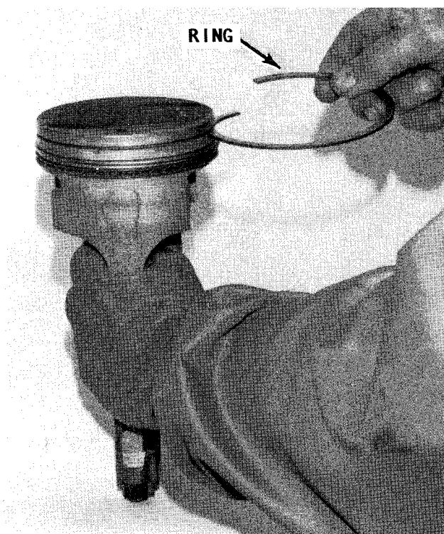
Proper installation of a new ring into the piston ring groove. Notice how the ring is bent slightly upward (left). After the ring is started, the ring is rotated around and over the top of the piston (right). The ring will feed into the groove and the end will finally snap into place.
