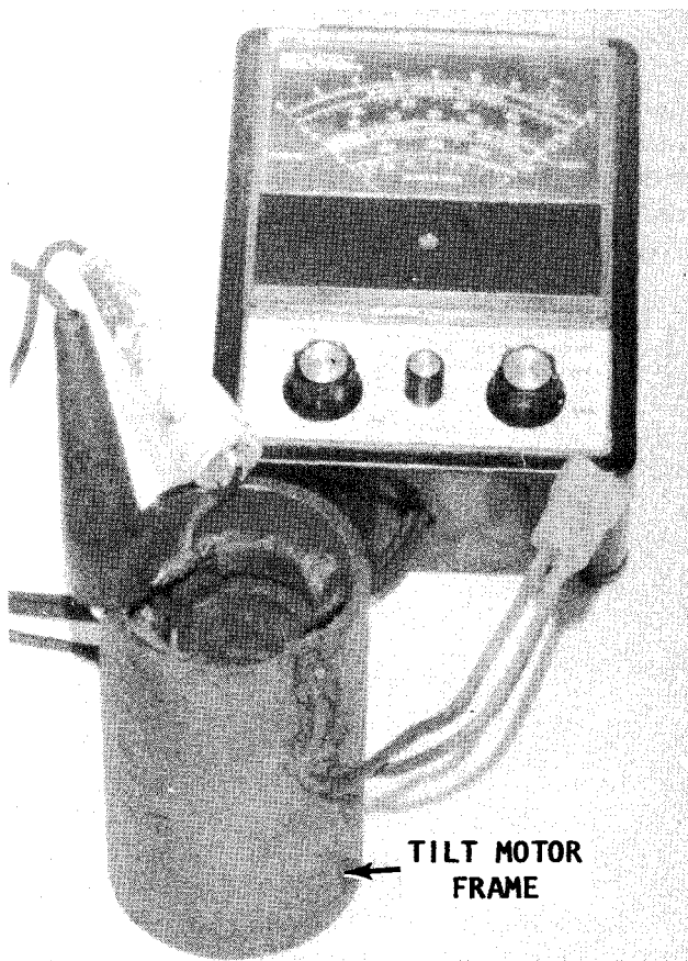
Testing the field coils, as described in the text.
