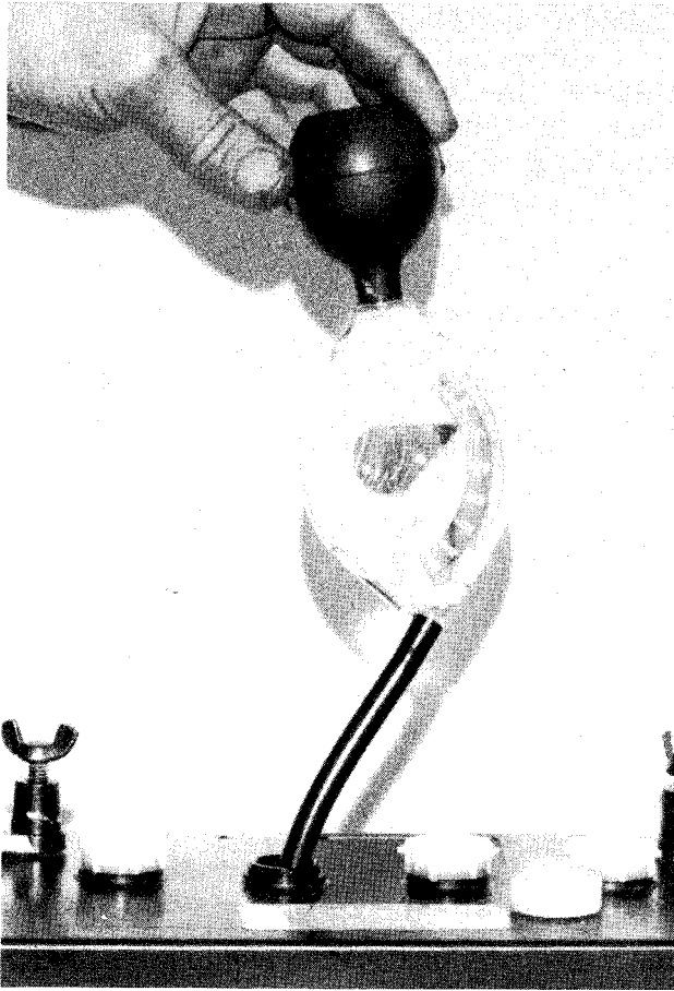
Test the battery electrolyte at regular intervals.
