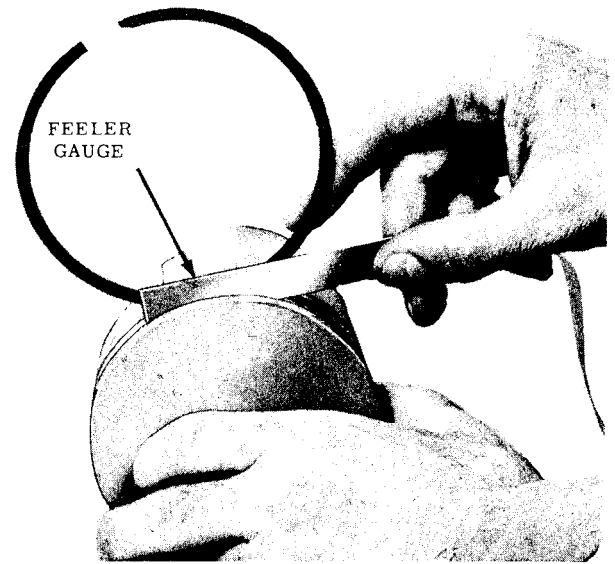
The piston-ring side clearance MUST NOT exceed 0.004".
