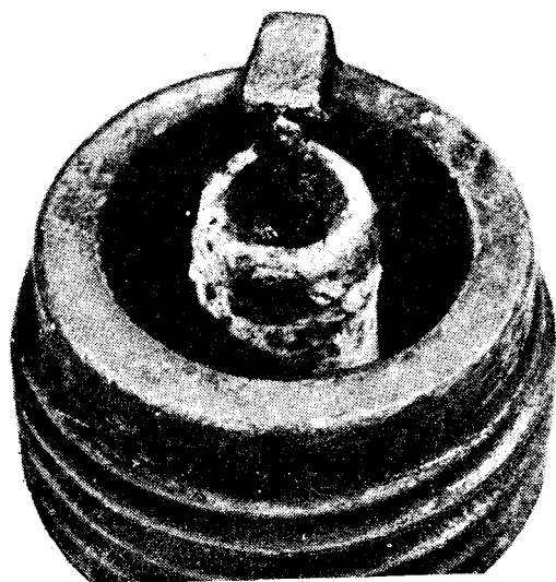
Ignition system defects will cause engine misfire. If the spark plug electrodes are improperly gapped, excessively worn, or corroded, the engine will misfire during acceleration.
