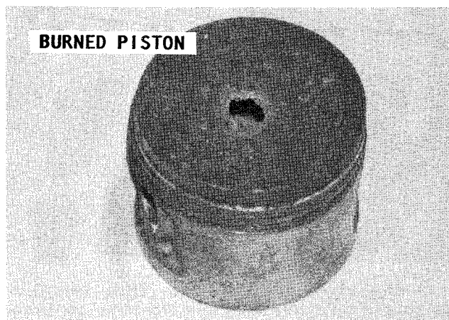
Preignition caused this piston crown to melt.
