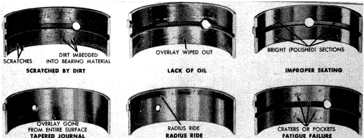
Examples of various wear patterns on bearing halves, including possible reasons for the condition.
