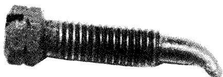
Tip of an idle mixture adjusting needle bent from being forced into its seat and against the closed throttle plate.
