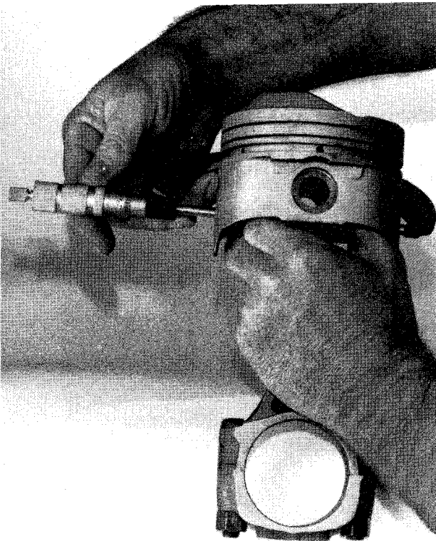
Using a micrometer to check the amount of piston wear.
