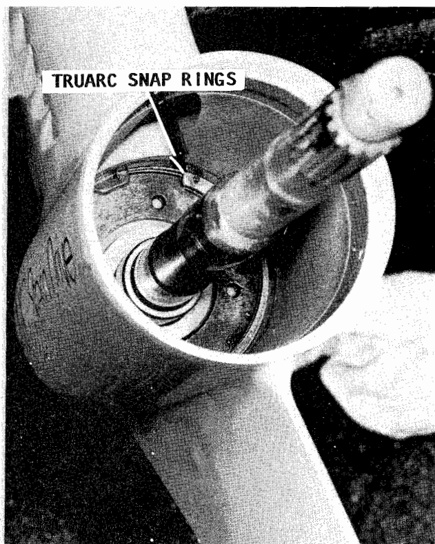
Truarc snap rings properly installed in the lower unit housing.
