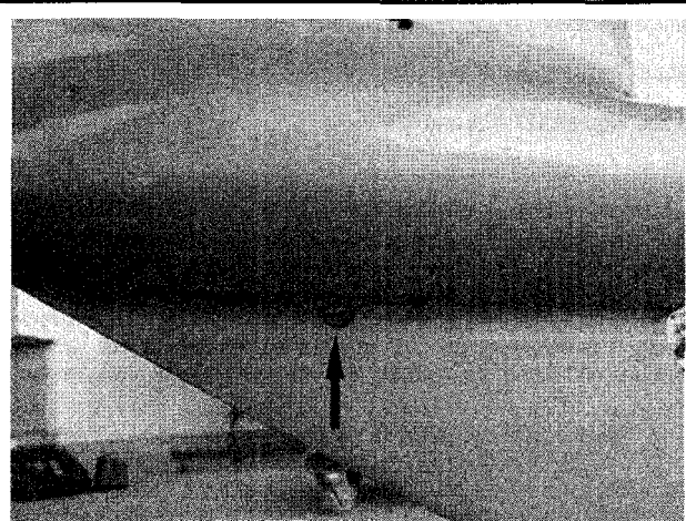
Fig. 129 The oil drain plug is on the port side of the housing
