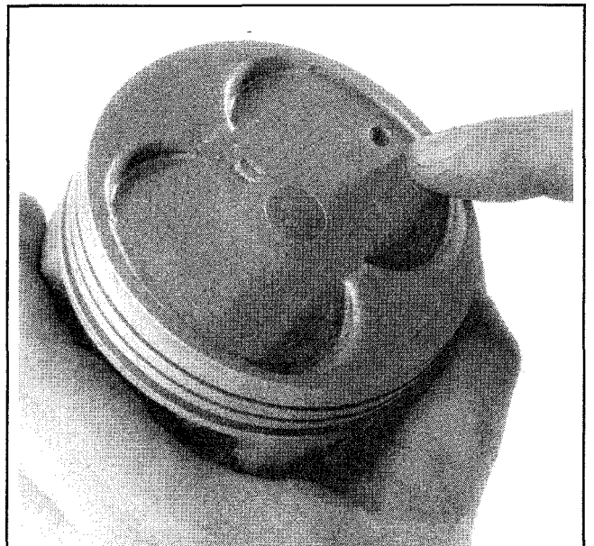
Fig. 54 Most pistons are marked to indicate positioning in the engine (usually a mark means the side facing the front)
