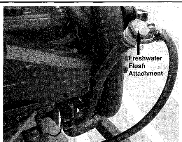
Fig. 107 Certain late model engines may be equipped with a fresh water flushing attachment (or have been retro-fitted), making it much easier to regularly flush your cooling system
