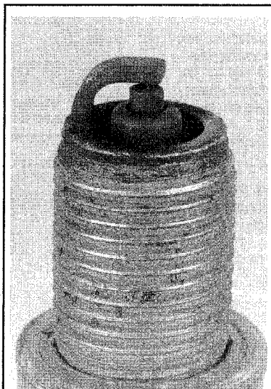
Fig. 63 A carbon-fouled plug, identified by soft, sooty black deposits, may indicate an improperly tuned engine
