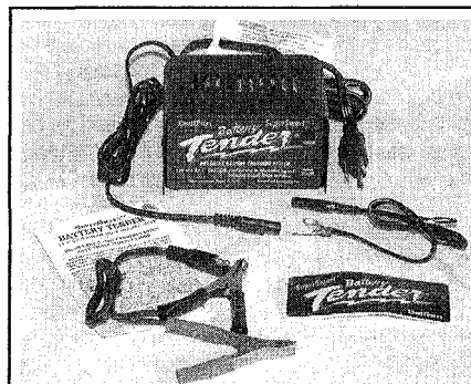
Fig. 27 Automatic chargers, such as the Battery Tender® from Deltran, are equipped with a sensing device to allow the battery charge to taper off to near zero as the battery becomes fully charged
