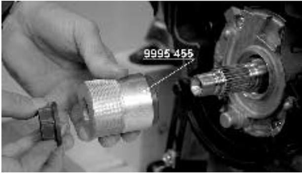
15. Install a new seal (1) on tool 9995455.
