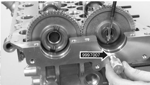
11. Put the lock pin 9997007 into the hole under the exhaust camshaft.
