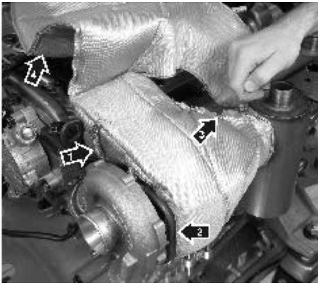
61. Insert the spring (1) from underneath between the turbocharger exhaust turbine and the vacuum capsule bracket. Hook the spring on. Make sure that the heat shield (2) goes in between the oil pipe and the exhaust turbine.
