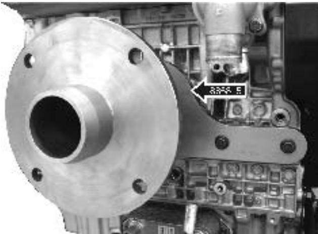
6. Install engine fixture 885815 on the engine.
