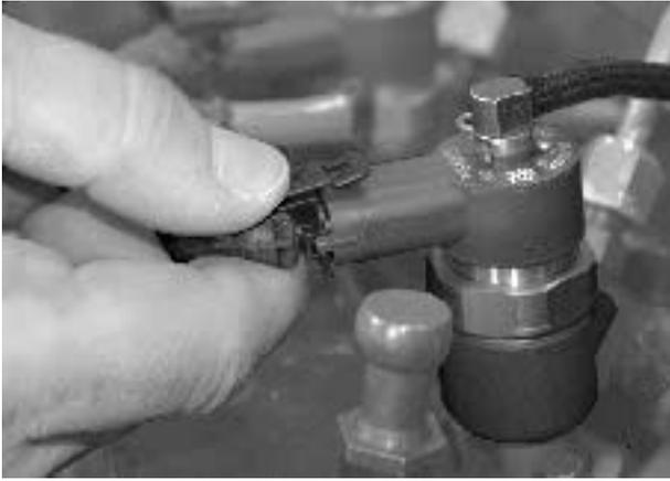
9. Undo the connectors for the injectors, and put the cable harness to one side.
