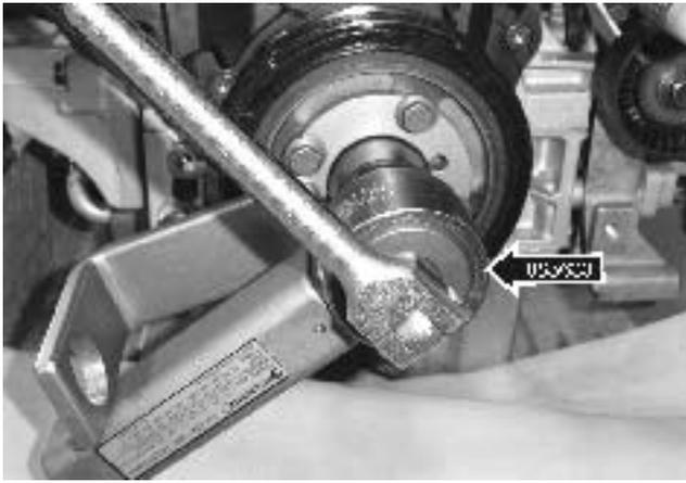
25. Install the torque amplifier (885633), together with 885648, as shown in the illustration.
