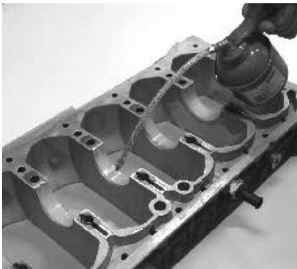
1. Put new main bearing shells in place in the engine block and joining piece, put a thin film of oil on the bearing surface.
