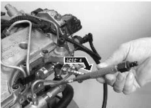
2. Start with no. 1 cylinder and install adapter no. 885814 in the tapped hole for the plug. Torque the adapter to 11 Nm. Connect compression tester 9988539 to the adapter.
