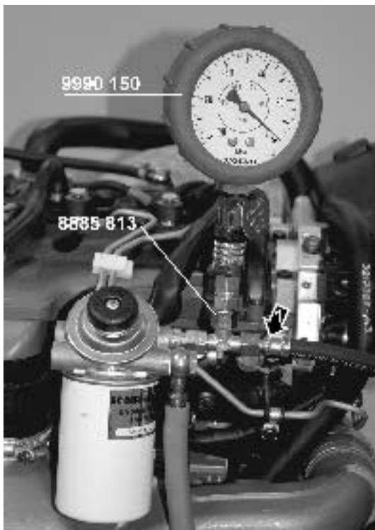
1. Unscrew the fuel union (1) on the fuel filter pump.
