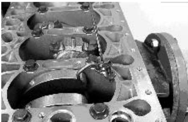
43. Remove the piston cooling nozzles. Rotate the crankshaft to access all the nozzles. Use magnetic pen, part no. 885822, to lift the nozzles out.
