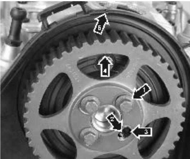
31. Fix the camshaft toothed belt pulley with one of the three screws (1). Check through the open screw hole (2) that the screws are not in their end positions in the elongated holes (3) on the toothed belt pulley. If the screws are in their end position, it may be impossible to tension the toothed belt.
