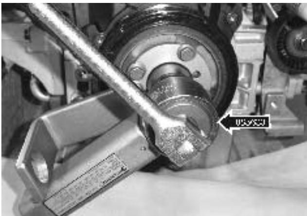
5. Install the torque amplifier (885633), together with 885648, as shown in the illustration.
