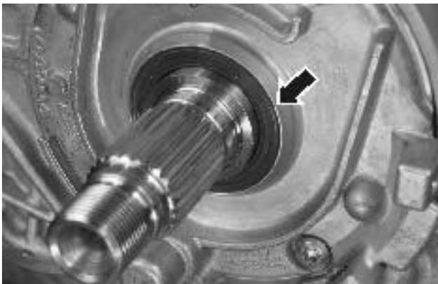
16. Check that the seal ring is level with the outer edge of the swage on the oil pump.
