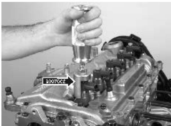
13. Remove the fuel injector pipes and the injectors.
