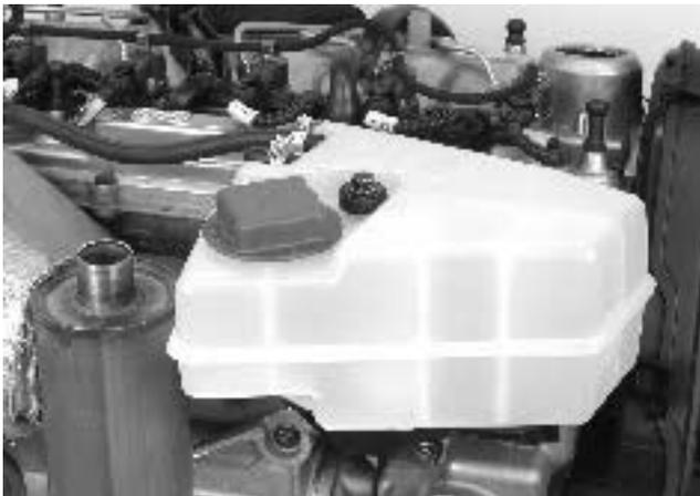
55. Install the expansion tank on its bracket.
