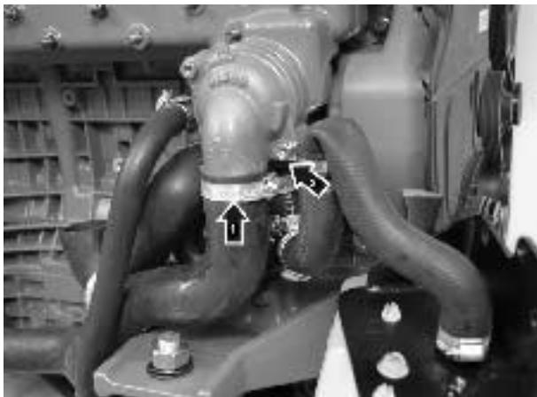
7. Remove the hose anchorage (1) on the thermostat housing and the inner hose connection (2) on the thermostat housing.
