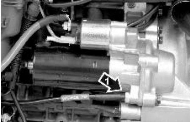
1. Undo all cables from the starter motor.
