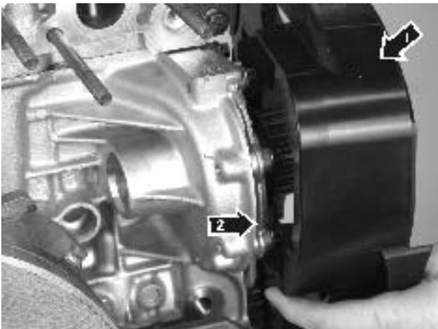
33. Install the rear timing gear cover (1). Check that it comes into the correct groove (2) behind the coolant pump.
