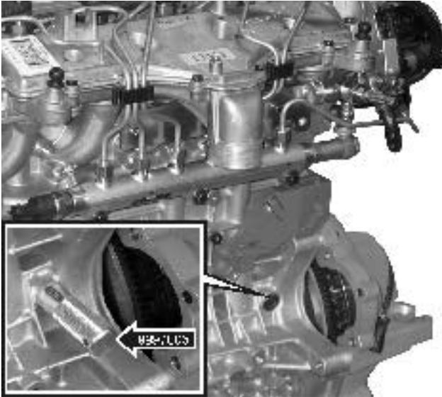
1. Unscrew the plug in the engine block and install locking pin 9997005 to lock the crankshaft. Make sure that the pin bottoms against the block.
