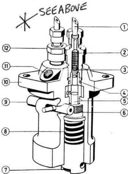
Fig. 49. Injection pump, D2 and MD2
