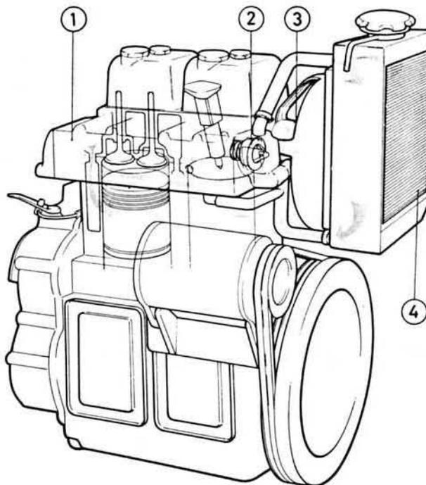
Fig. 67. Cooling system, D2
