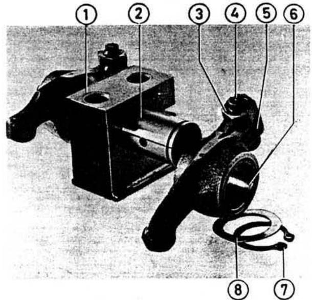
Fig. 17. Rocker arm mechanism
