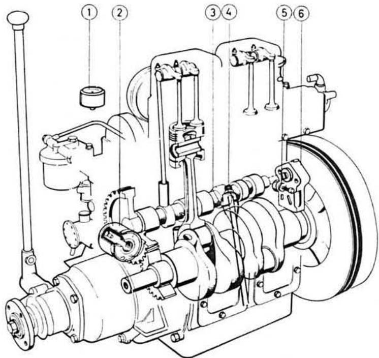
Fig. 39. Lubricating system, D2 and MD2
