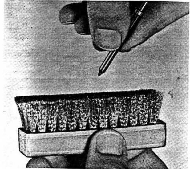
Fig. 54. Cleaning a nozzle needle
