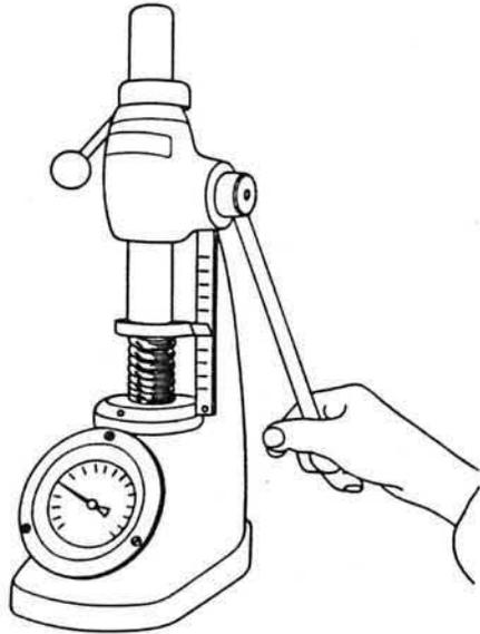
Fig. 16 Checking a valve spring.
