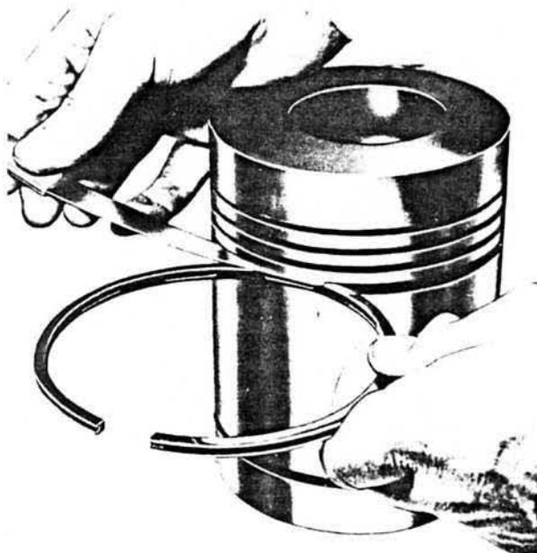
Fig. 24. Piston ring clearance in groove
