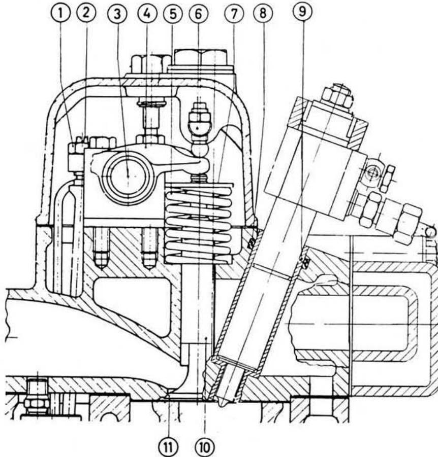
Fig 6. Cylinder head and valves
