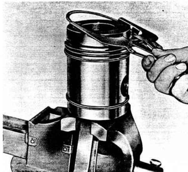
Fig. 25. Fitting the piston rings
