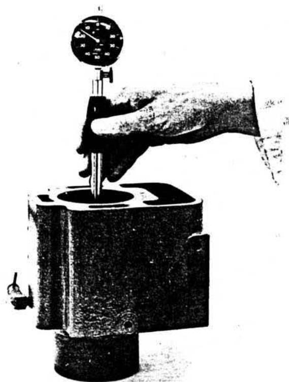
Fig. 21. Measuring cylinder bore wear.
