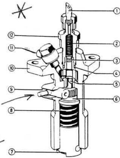
Fig. 48. Injection pump, D1 and MD1
