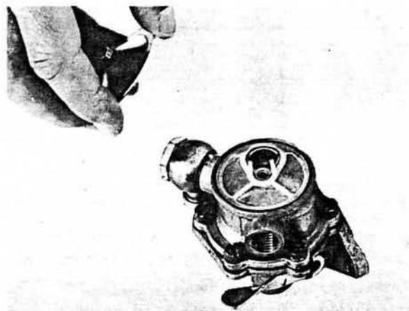
Fig. 64. Cleaning the strainer.
