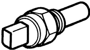
Fig. 124. Refrigerant temperature relay
