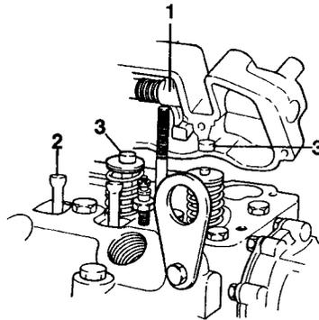
Fig. 32. Fitting of the rocker mechanism (MD2040)
