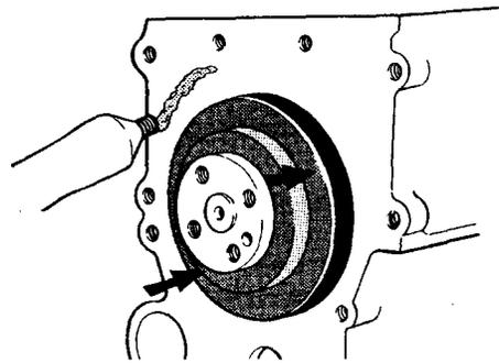
Fig. 81. Fitting of crankshaft seal
