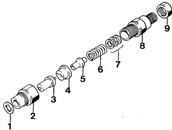
Fig. 86. Injector, complete
