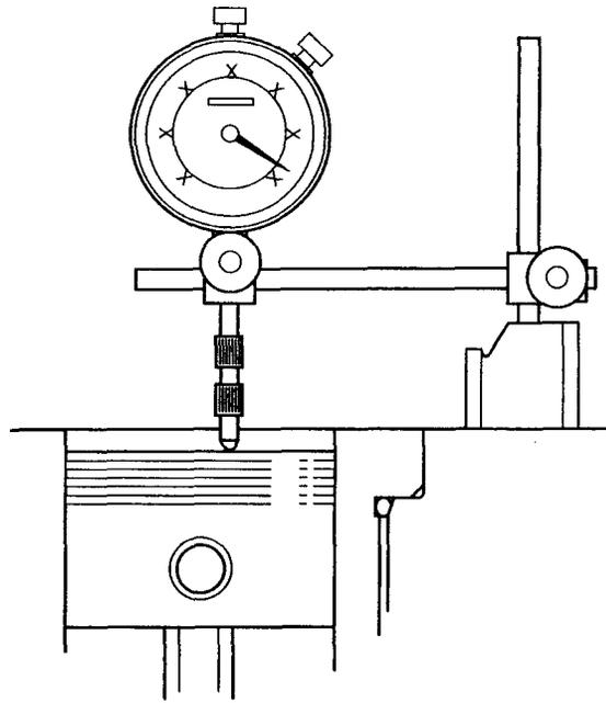
Fig. 91. Measurement of piston position with dial gauge
