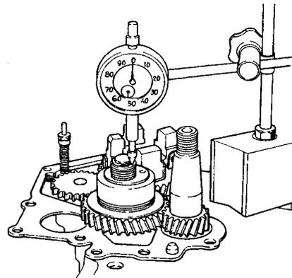
Fig. 63. Checking of oil pump's axial clearance
