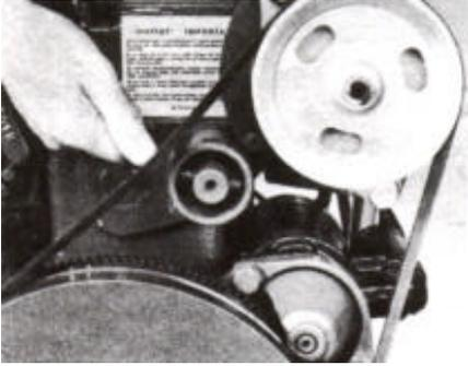
Check the belt carefully, both for wear and cracks. Any sign of such and the belt must be replaced. Loosen the alternator mounting bolts so that the belt can be removed. Clean the pulley grooves before fitting the new belt. Tension the belt so that it can only be depressed 5 mm (3/16") midway between the pulleys. After a few hours running, recheck belt tension and adjust if necessary.
