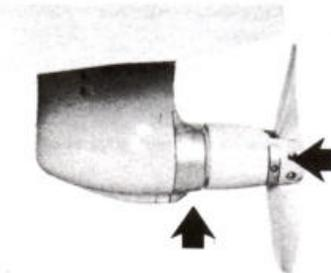
Replace the zinc-anode if it is eaten away to more than 50%. Remove the propeller and the spacer-ring with deflector and remove the Allen-head screws, holding the zinc anode. Clean the contact surface on the S-Drive and install a new zinc-anode. Be careful to obtain a good metallic contact between the S-Drive and the zinc-anode. Also replace the zinc-anodes on the S-Drive when eaten away to more than 50%. **NOTE!** Do not paint the zinc-anodes.
