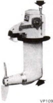
Remove the oil dipstick. Remove the plug underneath the propeller gear housing and let the oil drain off. Install the plug with its O-ring. Fill oil through the dipstick hole. The oil level shall be within the dipstick marks. NOTE! Do not fill oil above the upper oil dipstick mark. Concerning the choice of oil, see "Technical Data", Page 30.
