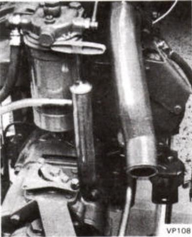
The oil can be drained from the reverse gear by removing the plugs under the reverse and reduction gears respectively (see Engine Component Guide), or by sucking up the oil through the dipstick hole with the help of an oil scavenging pump.
