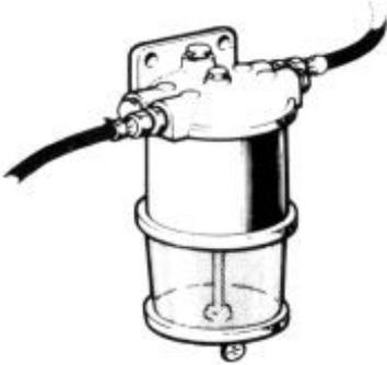
If an extra fuel filter with water separator is fitted, check the transparent bowl to see if there is any water in the fuel. If necessary, drain the filter via the cock in the bottom of the bowl. Try to avoid spilling fuel. Pump up the fuel and vent the system. The fuel filter element should be changed at least once a season.
