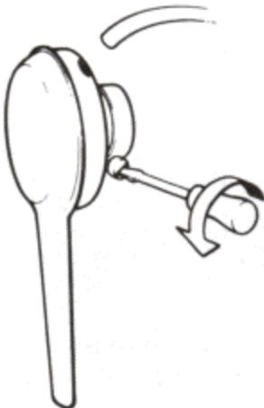
The air filter should be removed and cleaned after every 100 hours of operation or once per season.
