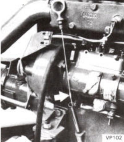
Each day before starting check that the oil level is between the marks on the dipstick. Top up with oil if necessary through the oil filler hole. NOTE. Do not top up above the MAX. mark. Concerning choice of oil, see under "Technical Data".
