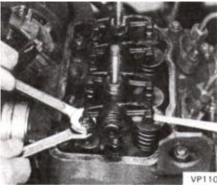
Checking and adjusting the valve clearance should be done by an authorized Volvo penta Service Workshop. See further under "Valves - Technical Data".
