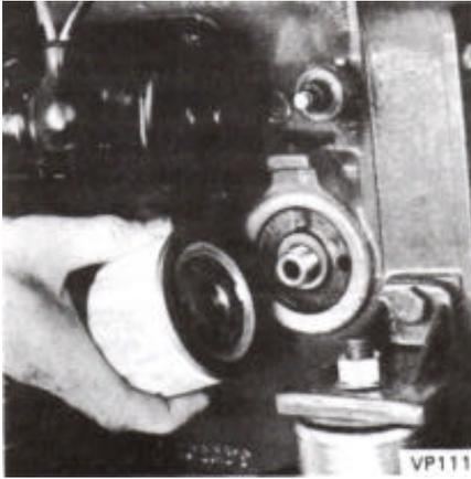
Coat the new oil filter's rubber seal with oil. Check the contact surface on the engine and screw on the filter by hand until it touches the contact surface. Turn the filter a further half turn, not more.
