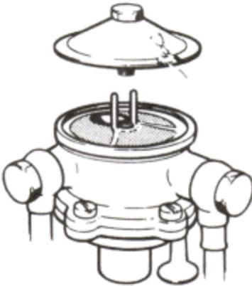
The fuel pump on the engine has a built-in strainer, which can be removed by removing the pump's cover. The strainer must be cleaned at least once per season. Always vent the fuel system. See "Venting of Fuel System" (page 23). **Check immediately after starting that there is no fuel leakage.**
