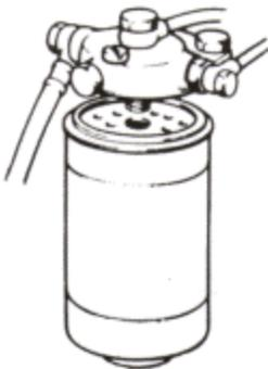
The fuel filter must be replaced least once per season. NOTE! If an extra fuel filter is installed in the boat, this filter or filter element must be replaced as well.
