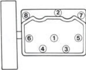
Retighten each nut **with a torque wrench** before starting a new engine or an overhauled engine for the first time, and then again after 20 hours of operation. The valve clearance should always be checked after the nuts have been retightened. Sequence for tightening nuts is shown in the figure opposite.
