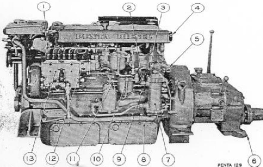
Fig. 1. MD 47 engine with Snow Nabstedt reverse gear.
