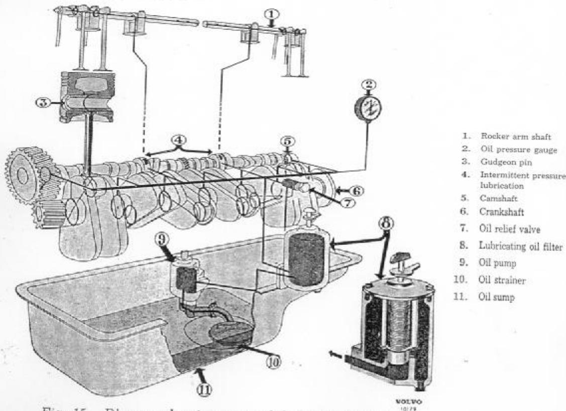
Fig. 15. Diagram showing engine lubricating system.
