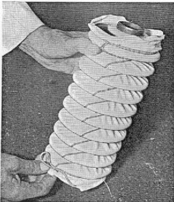
Fig. 20. The filter cloth fitted.
