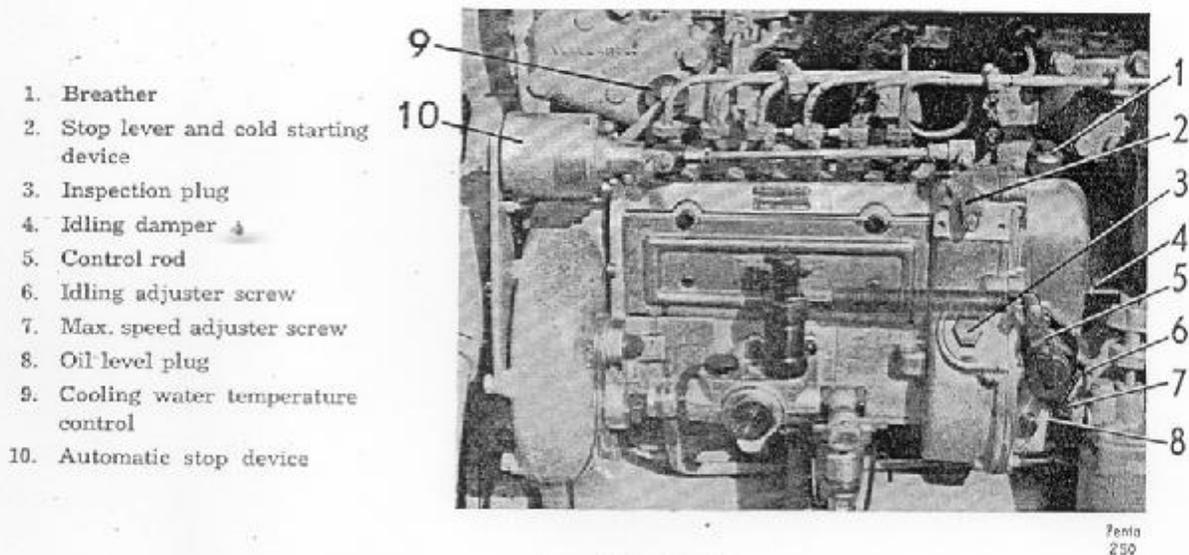
Fig. 34. Fuel injection pump with centrifugal governor C.A.V. (on MD 47).
