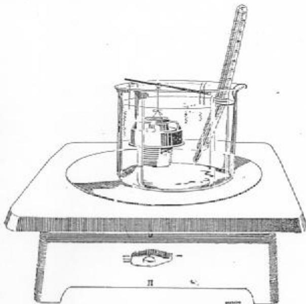
Fig. 43. Testing the thermostat.
