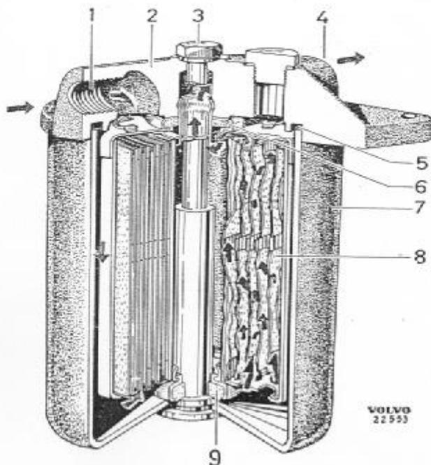
Fig. 27. Fuel filter, Bosch.
