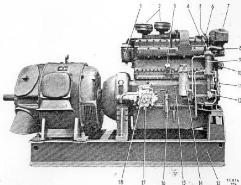
Fig. 8. MD 96 auxiliary unit with compressed-air starter motor.
