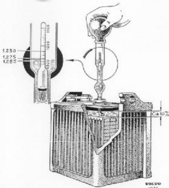
Fig. 46. Checking the specific gravity of the battery electrolyte and the electrolyte level.
