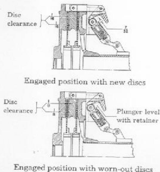
Fig. 51. Clutch mechanism.
