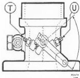
Fig. 35. Speed adjustment set-screws on throttle housing.
