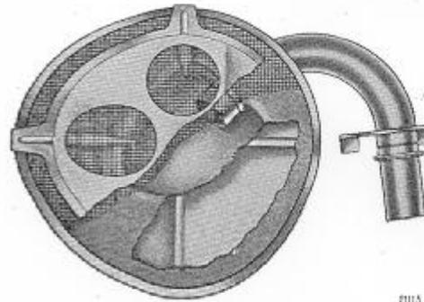
Fig. 21. Oil strainer, float type.
