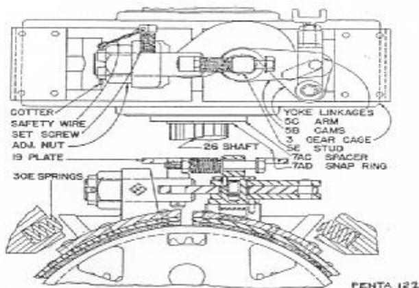
Fig. 52. "Astern" mechanism for MD 96 engine.
