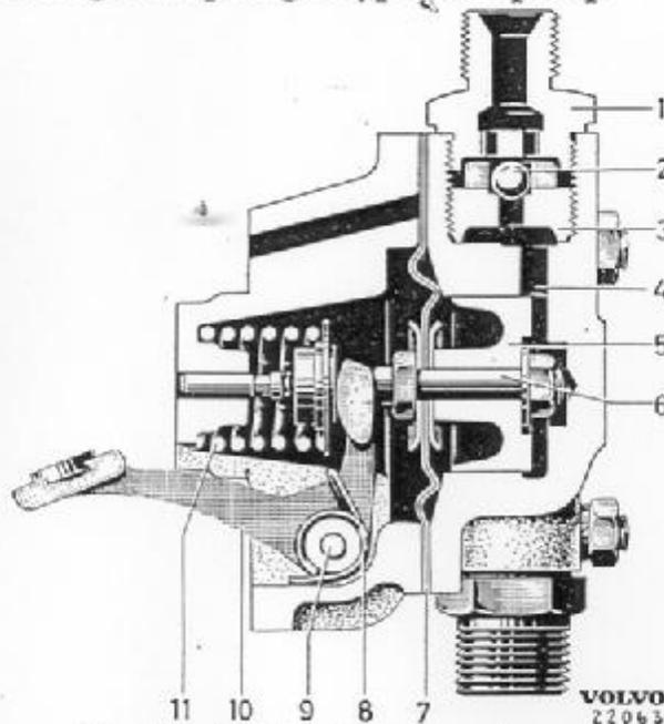
Fig. 25. Fuel feed pump, plunger-diaphragm type.
