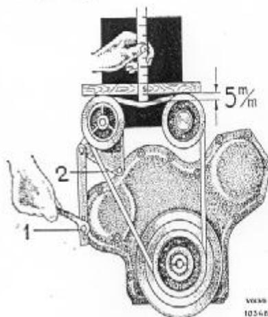
Fig. 45. Adjusting drive belt tension.
