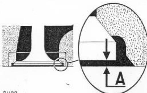
Fig. 13. The depth of the valve below cylinder head level.
