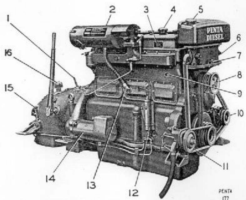
Fig. 4. MD 67 engine with Twin Disc reverse gear.
