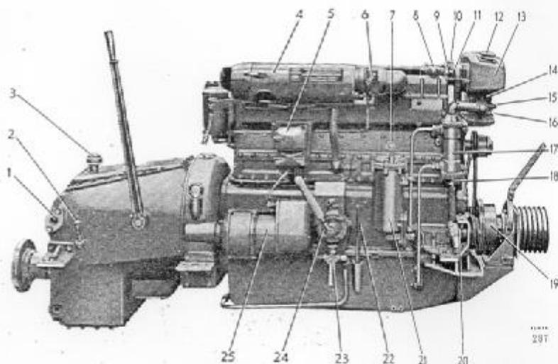
Fig. 6. MD 96 engine with Twin Disc reverse gear and Conax power take-off.
