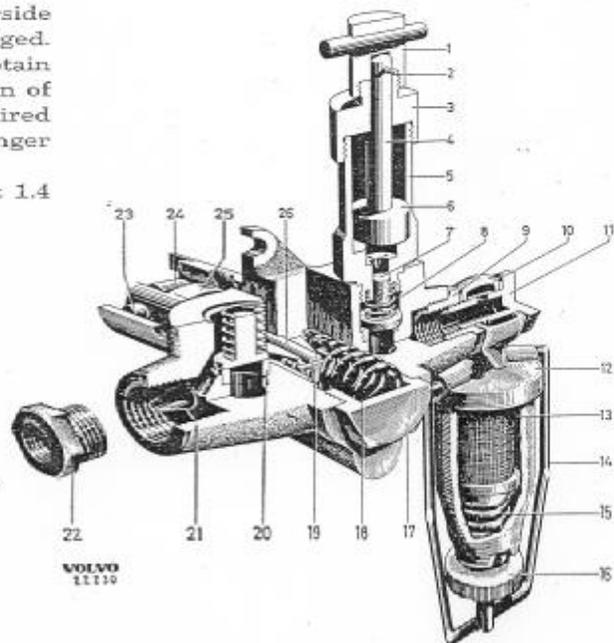
Fig. 24. Fuel feed pump, plunger type.
