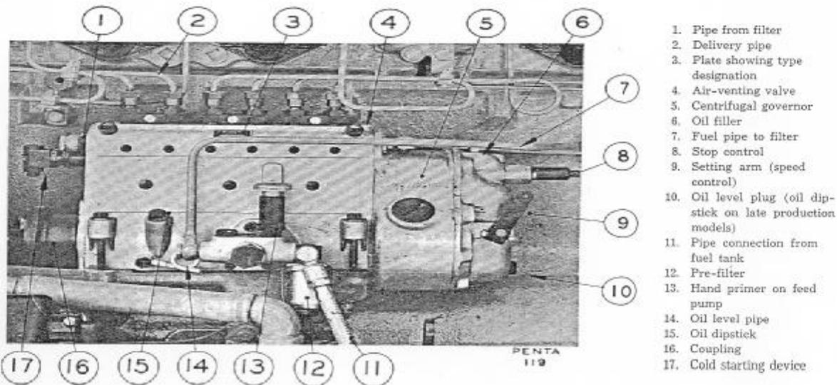
Fig. 33. Fuel injection pump with centrifugal governor, Bosch (on TMD 96).
