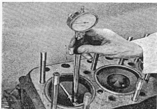
Fig. 11. Measuring the cylinder bore. Zero the indicator on the upper edge of the liner.
