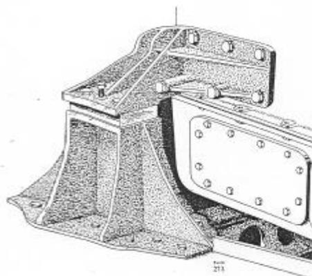
Fig. 69. Forward engine mountings.
