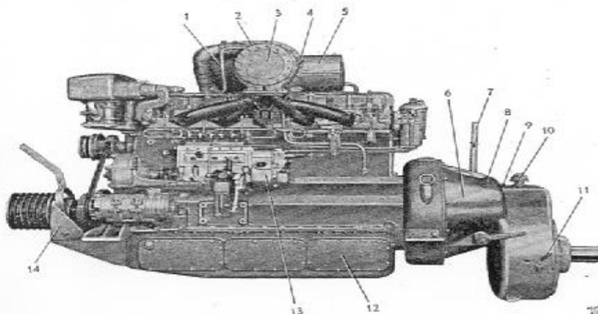
Fig. 7. TMD 96 engine with Twin Disc clutch and reduction gear as well as a power take-off with a Conax friction clutch.
