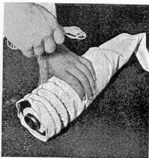
Fig. 19. Replacing the filter cloth.
