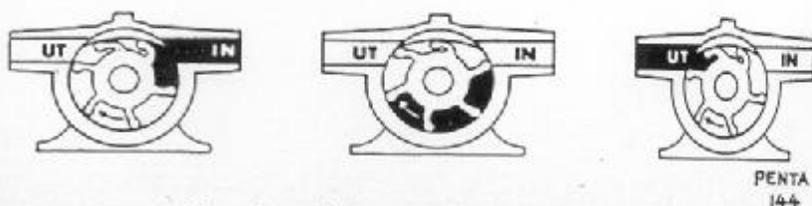
Fig. 44. Function of sea water pump.
