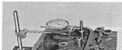
Fig. 12. Checking the clearance the valve stem and valve guide.
