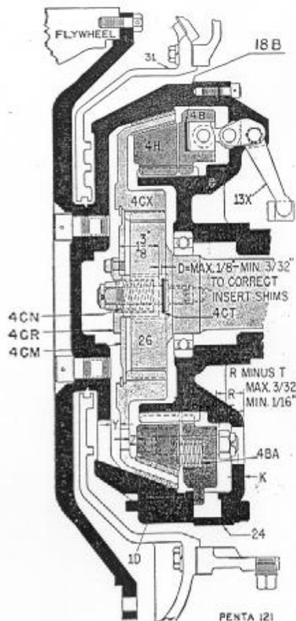
Fig. 53. "Ahead" mechanism for MD 96 engine.
