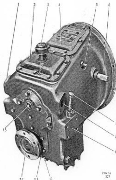
Fig. 50. Twin Disc reverse gear with reduction gear for MD 67 engine.
