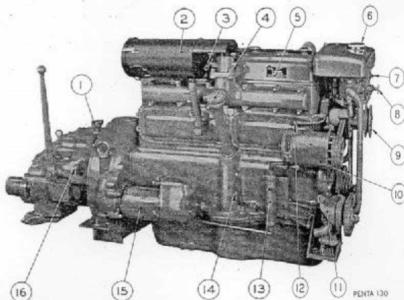
Fig. 2. MD 47 engine with Snow Nabstedt reverse gear.
