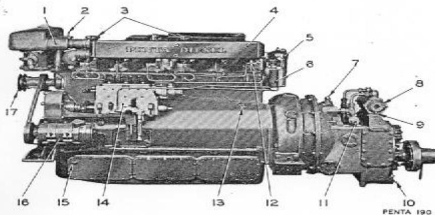
Fig. 5. MD 96 engine with Self Changing Gear reverse gear.
